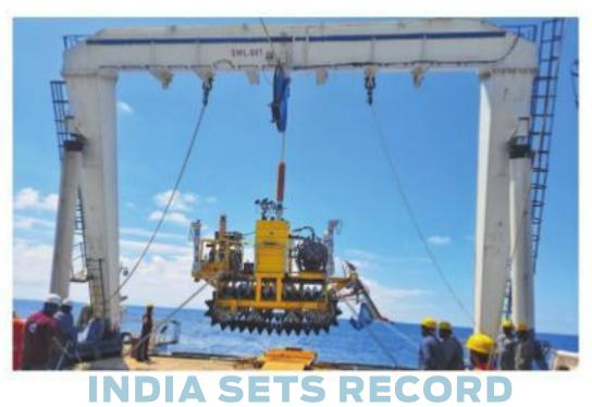
The scientific crew from the Chennai-based National Institute of Ocean Technology created history this April by conducting the world's deepest underwater locomotion trials — at a depth of 5,270 m — of an indigenously-developed seabed crawlerbased mining machine in the Central Indian Ocean Basin I SPECIAL ARRANGEMENT
